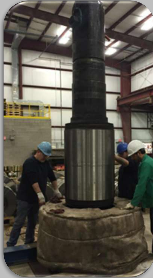
Arbor being carefully lowered into pre-heated sleeve.
